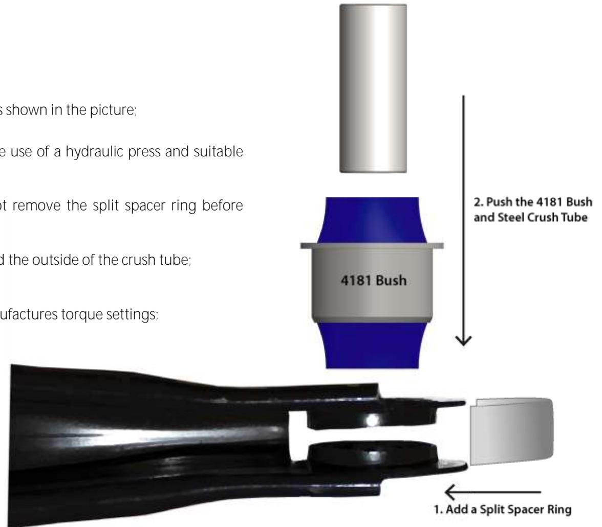
*Note:* Polyurethane bushings must be fitted to both sides of the vehicle. This kit should be installed by a Qualified Motor Mechanic.
