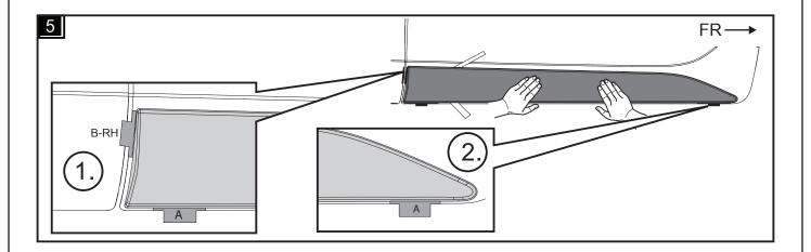
5. Place the front door mould onto door panel, aligning it to the sticker templates. Apply firm pressure to part in position 1 to door panel and then check level of part in the portion between sticker templates A. Apply firm pressure to part in position 2 to door panel.
