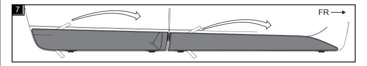
7. Open doors to full opening angle to ensure moulds do not interfere with body panel. Remove the remaining release liners in the direction according to Fig. 7. Check all release liners have been removed as failure to do this may cause the product to drop off or peel off. Then apply pressure force of 49N ±1N on all areas of the part with double-sided tape. Failure to do so may cause product to drop or peel off. Remove all sticker templates.
