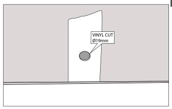
Drill/cut headliner at marked location using a 19mm vinyl cutter. Repeat for opposite side.
