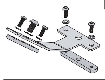
Secure the anchor plates to the cover plate using the M6x16mm button head bolts, M6 spring washers.
