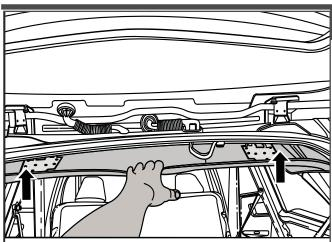
Lower headliner carefully to allow access to rear closure hinge fasteners.
