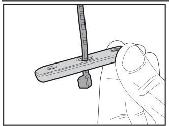
Insert a large cable tie through the centre hole of one of the anchor plates as shown.
