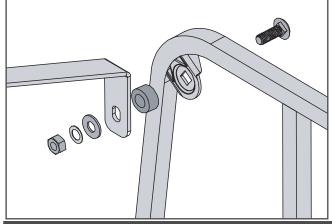
Fasten the rear top straps to the barrier using the M10 coach bolt, spacer, flat washer, M10 wave washer and M10 hex nut.
