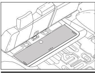
Remove large grommet from centre of floor pan and follow instructions on the 'Floor Pan Drilling Template' to align it across vehicle floor.
