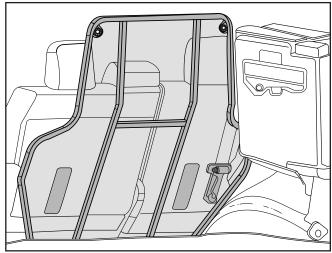
Install barrier through the rear vehicle.
