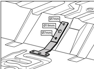
Place the lower cover plate on the floor pan and align with the drilled holes.
