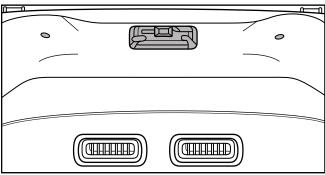
Using a trim removal tool, dislodge and remove the rear interior light and two rear headliner trim plugs.
