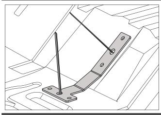
With the anchor plates below the floor pan, place the lower cover plate on the floor pan and feed the cable ties through the larger centre holes in the plate.
