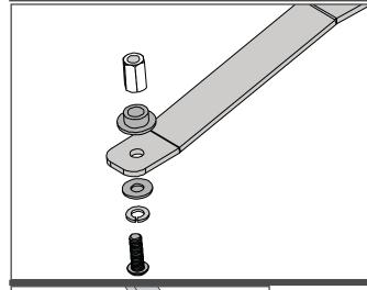
Fasten the rearward end of the top strap to the pre installed mounting points using the 7mm plastic bush, M8 flat washer, M8 spring washer and the M8X25mm Button Head Bolt
