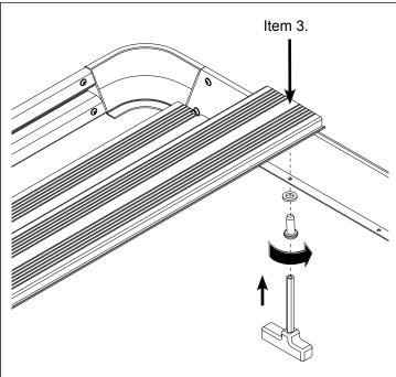
Remove both rubber buffer strips and all four end caps.
