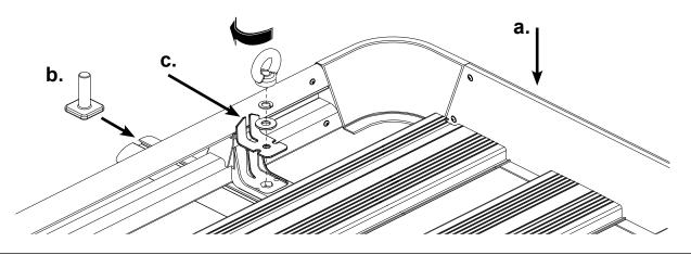
Adjust the alloy tray on the cross bars so that; All dimensions marked 'a' are equal. All dimensions marked 'b' are equal also. Tighten the eye nuts to secure the alloy tray to the cross bars. Ideally the eye nuts should be sit parallel to the cross bars when tight.
