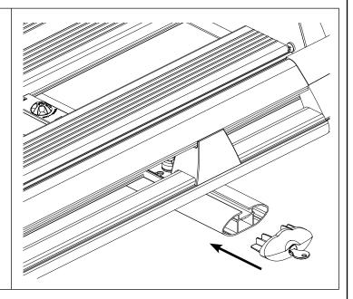
Re-fit the rubber buffer strips into the top of the cross bars if the alloy tray is removed.
