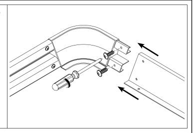
Attach the plank extrusions to the front and rear rails extrusions. Fasten each plank with two M6 security bolts and two spring washers using the allen key provided.
