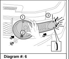
6.To complete installation, insert the top clip between the headlamp assembly. Position the bottom slot over the metal clip aligning the hole in the clip with the slot in Headlamp Cover, press down over the metal clips and at the same time apply upwards pressure to Headlamp Cover. Then secure the Headlamp Cover with screws and washers provided. **See Dia #6**.
