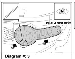
3. Trial fit the Headlamp Cover centrally on the headlamp by carefully locating the top clip under the headlamp assembly. Note the slot in the bottom of the Headlamp Cover and the dual lock-discs. Mark these locations onto the headlamp assembly with a non-permanent marker. Remove the Headlamp Cover. **See Dia #3.**
