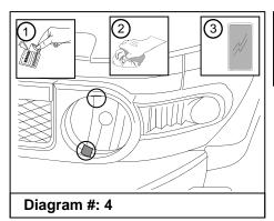
4. At the previously noted and marked slots positions, clean the headlamp lens with the alcohol wipe provided. Remove any residue with a clean dry cloth. Adhere the abrasive resistant tape strips provided to the cleaned areas. **See Dia #4.**
