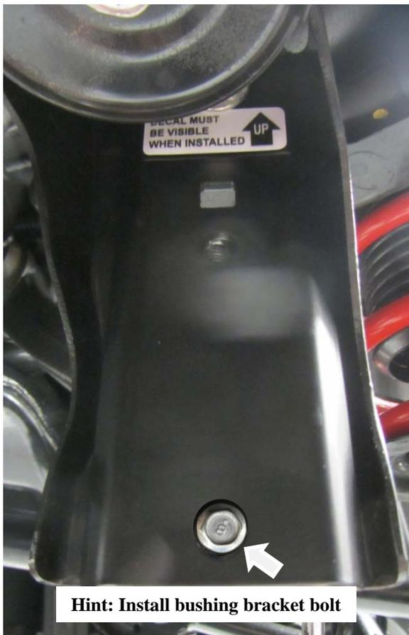
**Hint: Install bushing bracket bolt**
