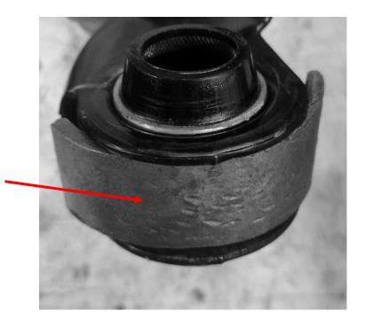
'C' piece used to support the arm while pressing.
