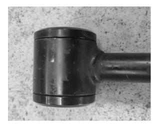
• Grease the bore of the bush and the outside of the crush tube and then push the crush tube into the bush, the assembled bush should look as below
