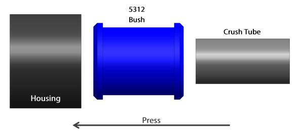
Note: Polyurethane bushings must be fitted to both sides of the vehicle. This kit should be installed by a Qualified Motor Mechanic.
