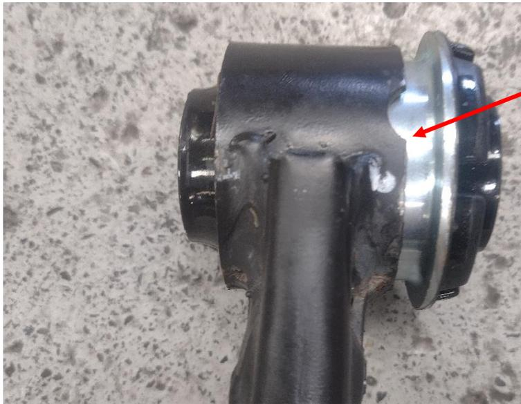
5mm gap between the underside of the flange and the outer face of the arm
