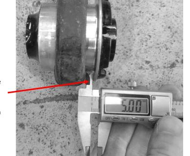
5mm gap between the underside of the flange and the highest point on the outer face of the arm (same for both bushes)
