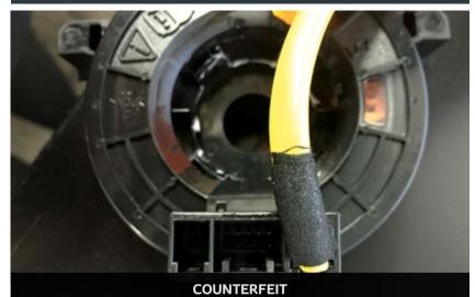
An Airbag Spiral Cable provides the wiring connection that allows an electrical signal to be sent to the driver's airbag for deployment.
