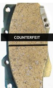
This counterfeit brake pad contains asbestos, posing a major health risk to automotive technicians and the general public when the brake pad material wears and creates dust.
