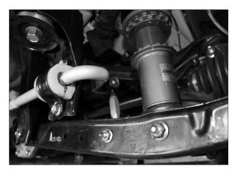
Place spacers either side of link for OE swaybar or 'middle setting' on adjustable swaybar.
