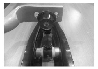
• Place spacers towards front side of control arm for hard setting on adjustable swaybar.
