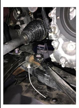
Note - some models will require the removal of the side engine mounts - to access the front bushing bolts
