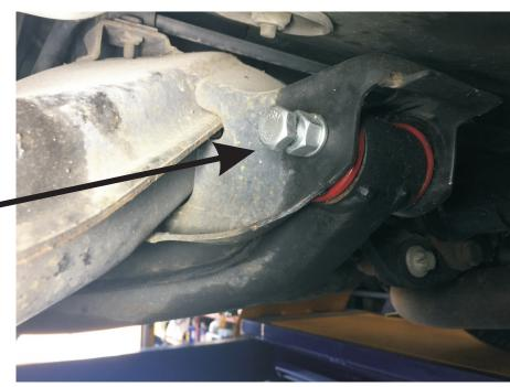
Place 50mm adjuster bolt on bushing side with best access for live adjustment.
