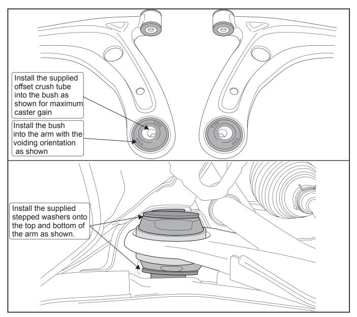
□ Install steel shell bush into the eyelet of the arm so that the bush is centralised in its position.
