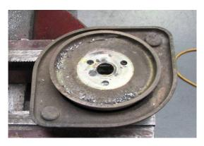
7. Separate the upper part of the strut top from the bottom washer by holding the drilled strut mount in the vice and using a chisel to gently separate the two sections (as per diagram B)
