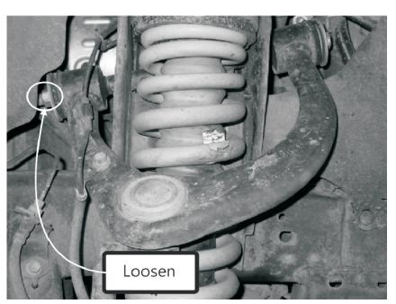
Note: Removal of the mounting bolt will require the removal of the batteries.
