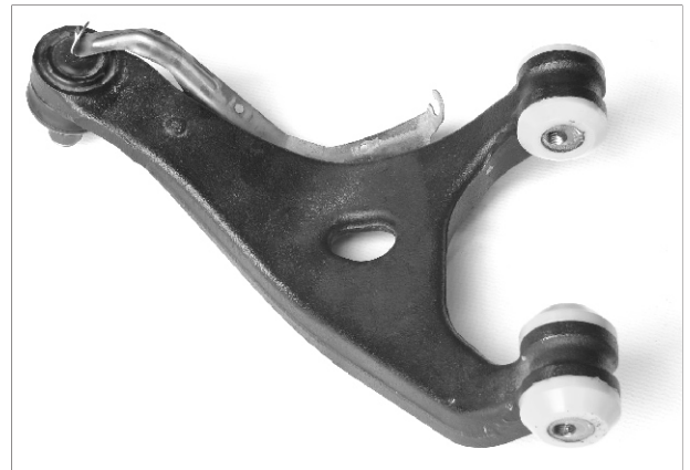
Fig 2 - left control arm with new bushes.
