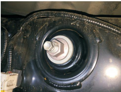
7. Re-use original washer and flange nut - tighten to 80 Nm.
