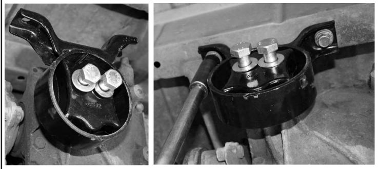
4. Clean the ID of the housing making sure it is free from any rust or burrs and insert the new bushing into the housing as per fig. 4.
