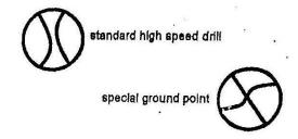
2) Grind a standard high drill flat nosed like a mill cutter – then backflute the two spirals to a razor sharp edge.
