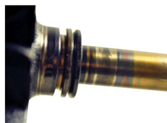
High temperature and material transfer to bearing.
