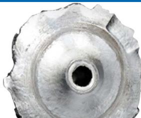
Orange peel effect on back face of compressor wheel is a clear sign of overspeeding.
