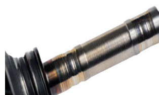
Worn and scored bearing. Material transfer to the shaft.
