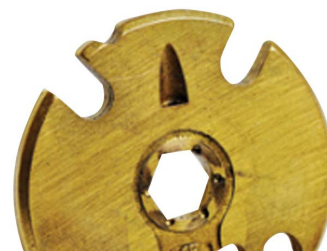
Large particles in oil can cause deep scoring and impacts.
