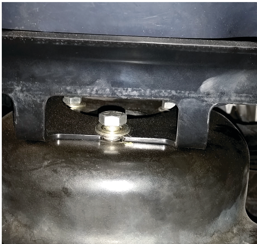
Figure 3: External reservoir mounting bracket
