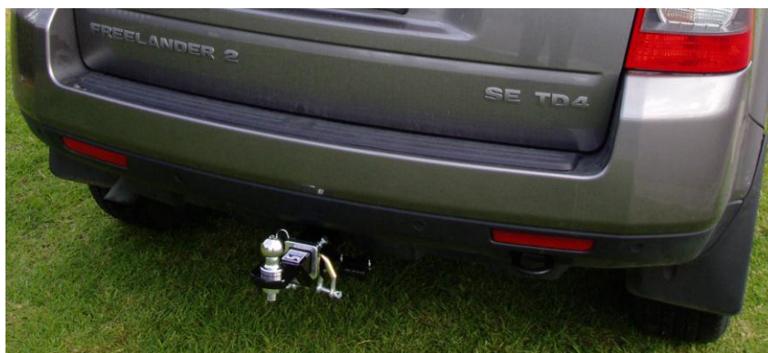
Figs 6 install towbar between towing hook and chassis rail.
