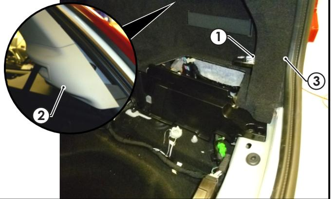
7. Dislodge the upper section of the lower trim and then disconnect the RHS tail light connector (1) and then patch the trailer patch (P/No: 101443-WL) (2) in between.
