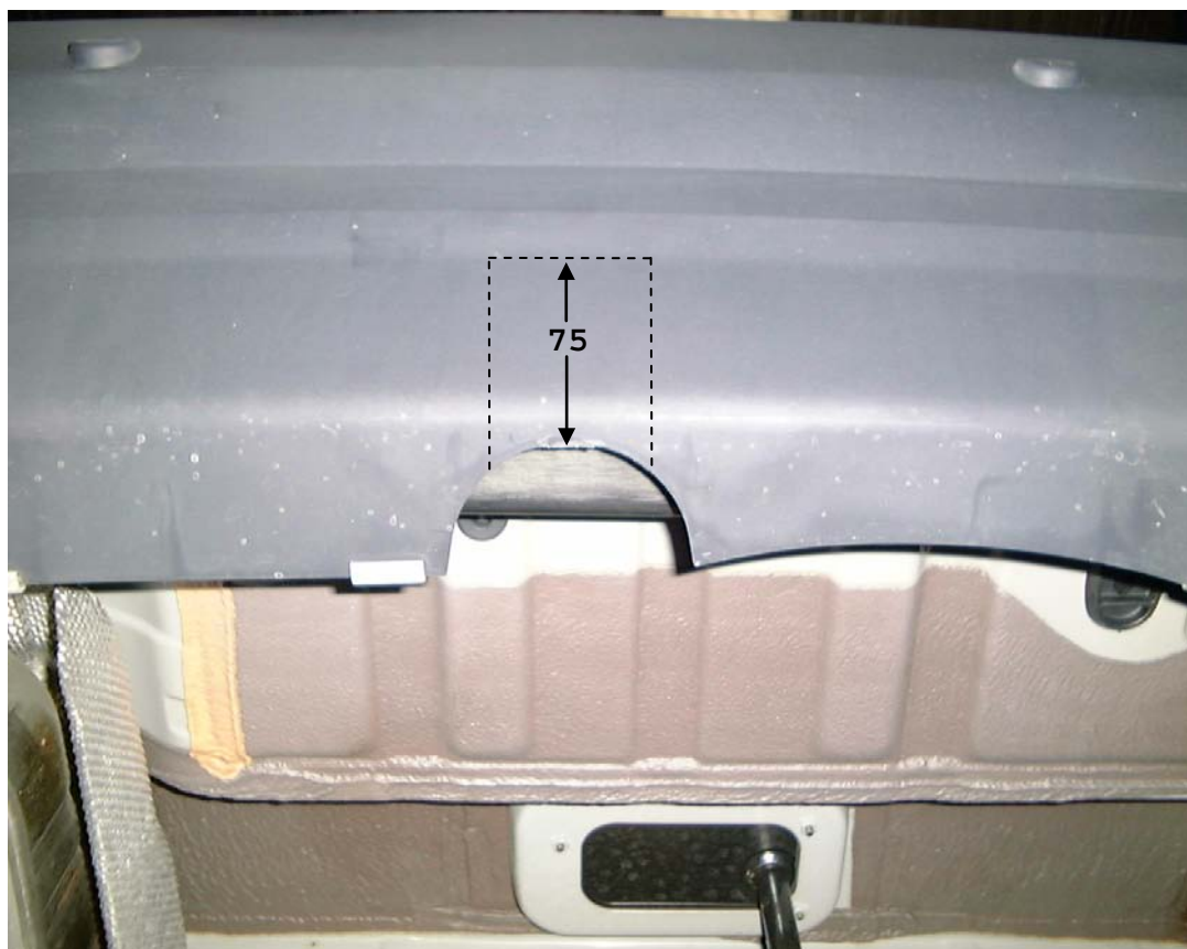
Bumper cut diagram 2, 75mm to be measured around the outside of the bumper.
