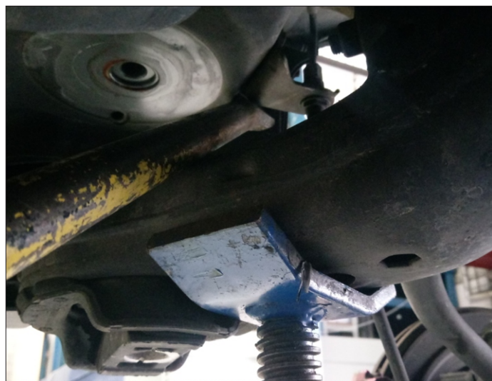
Figure 03 - Lowered Cradle being moved back for
