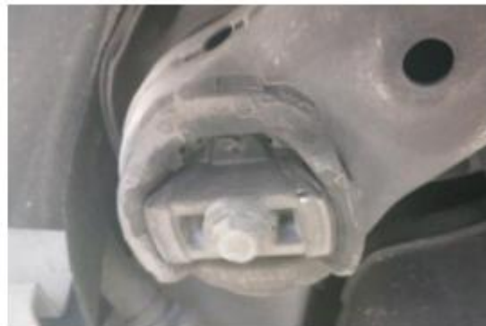
Figure 02 – Cradle Bolts to be loosened.
