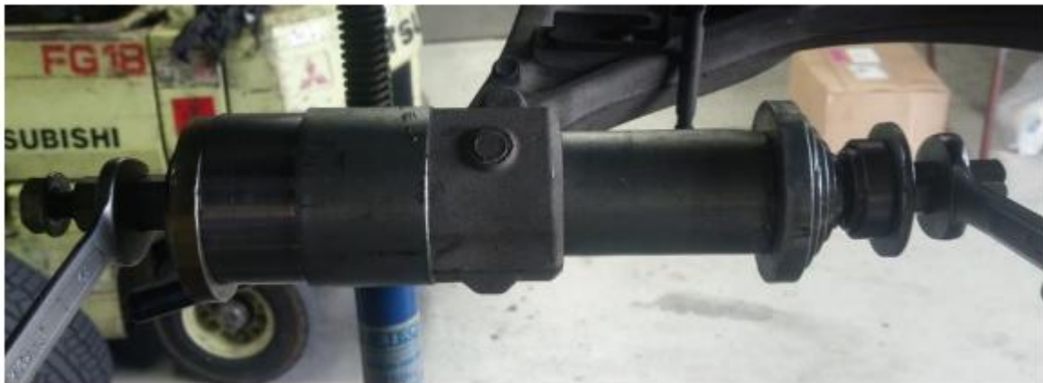
Figure 04 – Booker-Rod set up to remove pre-existing bushes.
