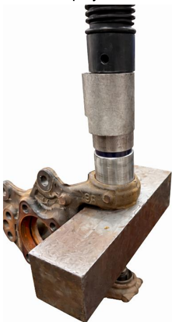
Figure 7- Bush installation using press and suitable press tools.
