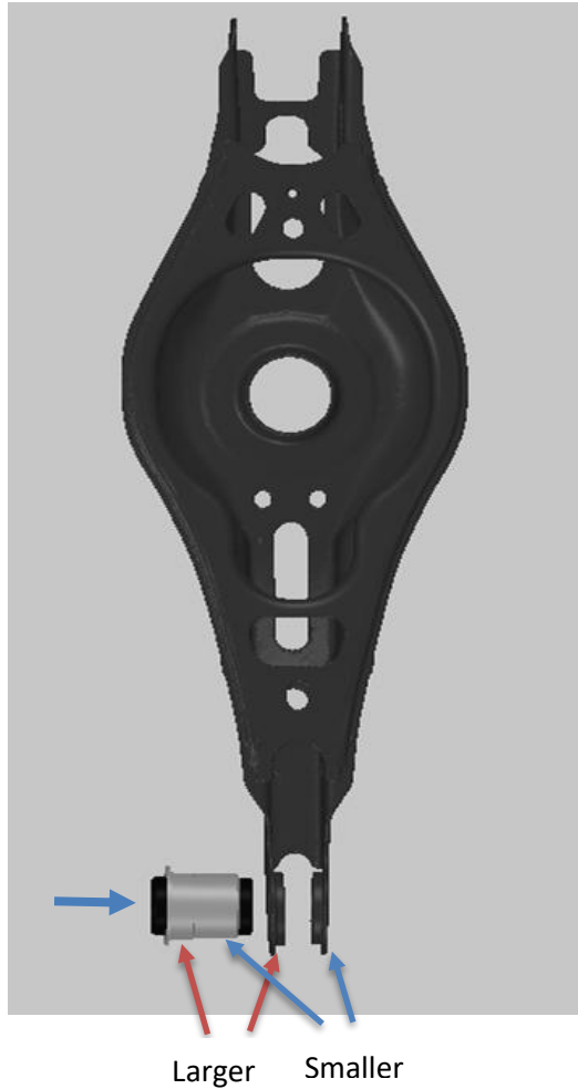
Figure 3: Direction to push in new polyurethane bush
