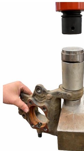
Figure 5- Example of bush positioning in press.
