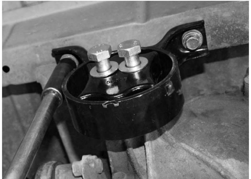
4. Clean the ID of the housing making sure it is free from any rust or burrs and insert the new bushing into the housing as per fig. 4.
