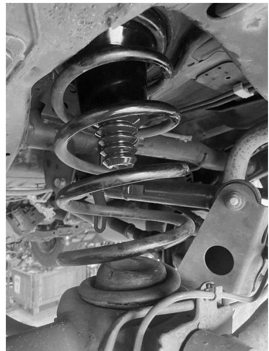
Figure 01 – Completed Installation of Bump Stop
