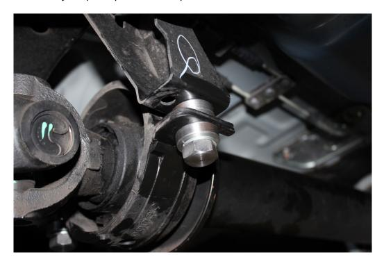
Diagram shown below is the start out position to eliminate vibration. Adjust as necessary.
