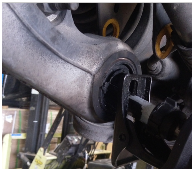
Figure 03 - Removal of Shock Eye Bush
