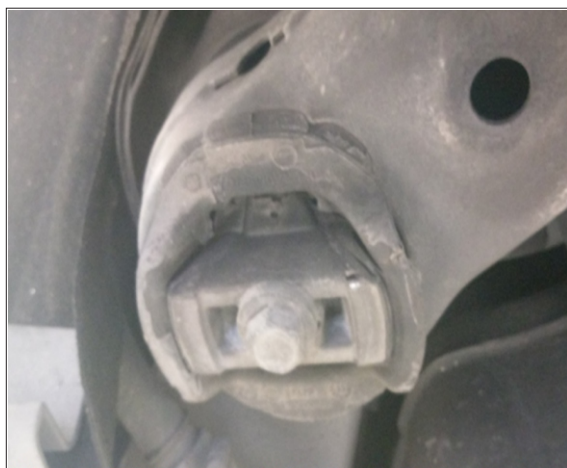
Figure 02 - Cradle Bolts to be loosened.
