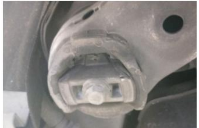
Figure 02 – Cradle Bolts to be loosened.
