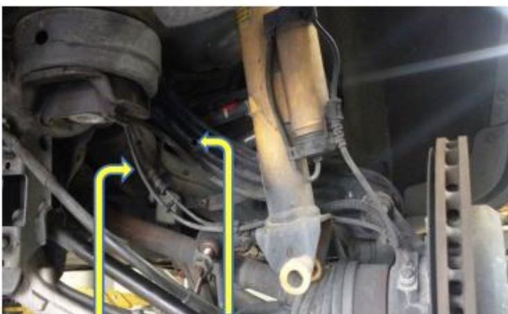
Figure 03- Wiring system to be freed from right rear upper control arm.
