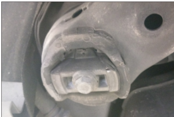
Figure 02 – Cradle Bolts to be loosened.
