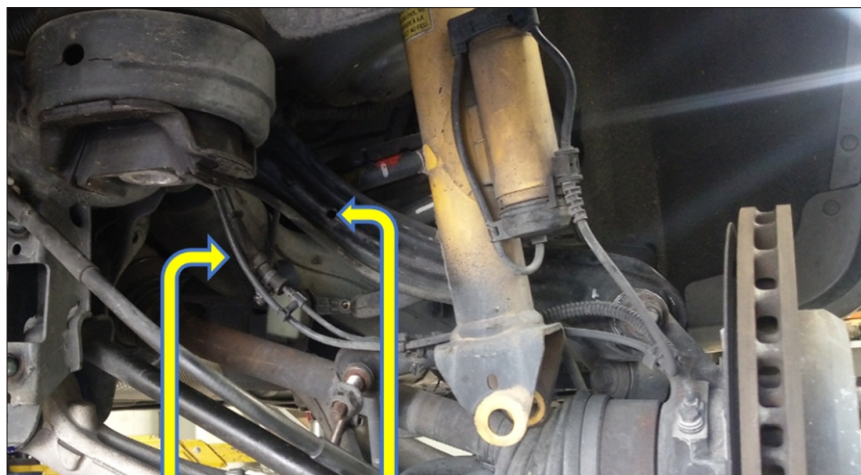
Figure 03- Wiring system to be freed from right rear upper control arm.
