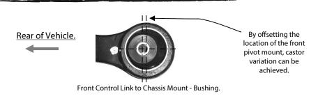
Note: Polyurethane bushes must be fitted to both sides of the vehicle.
