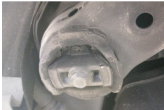
Figure 02 – Cradle Bolts to be loosened.
