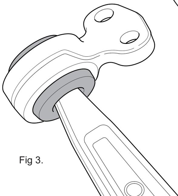
3. Offset bush to be installed as per Fig 2.
