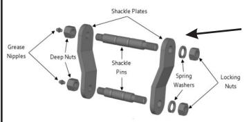
Assembly image of rear shackles. Note - do not over tighten grease nipples
