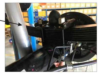
Remove old bushings from leaf spring and chassis
