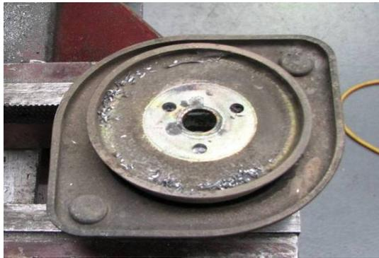
7. Separate the upper part of the strut top from the bottom washer by holding the drilled strut mount in the vice and using a chisel to gently separate the two sections (as per diagram B)
