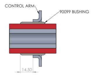
PRESS SUPPLIED BUSHING INTO THE CONTROL ARM, LEAVING 14.5mm OF THE STEEL SHELL PROTRUDING FROM THE OUTER EDGE OF THE ARM
