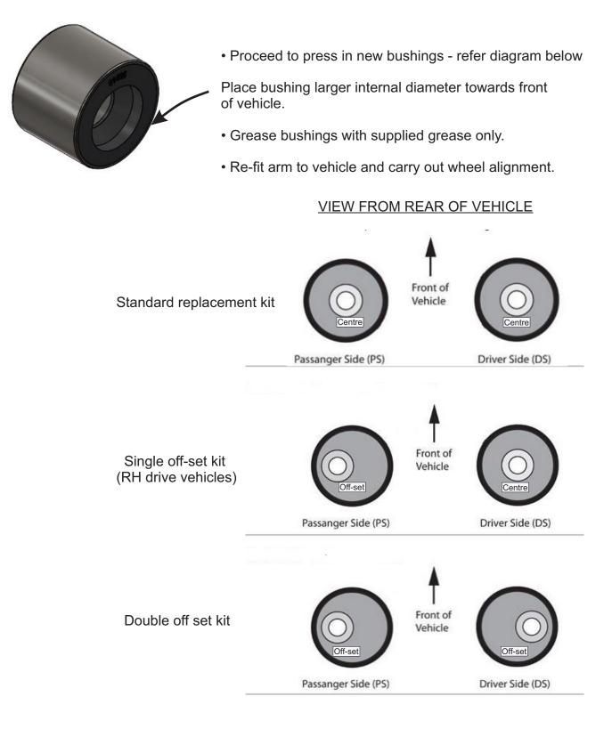
It is recommended that a licenced workshop or tradesperson carry out the above procedure and that workshop manual and relevant safety procedures are followed in addition to the above.
