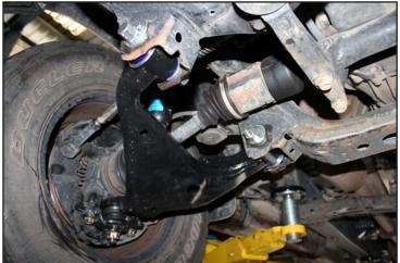
• Lightly grease new bushing side faces with supplied grease.
