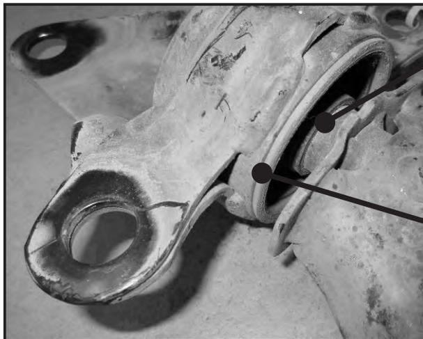
PRESS OEM BUSHING OFF THE CONTROL ARM SPIGOT ENSURING NOT TO DAMAGE THE RUNNING FACE.
