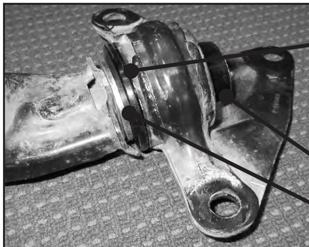
LUBRICATE WASHER THRUST FACE AND BUSHING BORE WITH SUPPLIED LUBRICANT.
