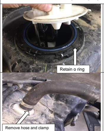
Remove the fuel sender from the tank, retain the sender and the o ring for the installation process.
