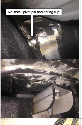
When the tank is in position install the pivot pin and spring retaining clips to eyelet in the strap and the original point in the chassis.
