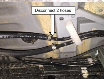
Disconnect the supply and return hoses from the steel fuel lines at the LHF corner of the fuel tank.
