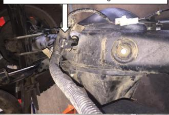
Loosen the bolt securing the wiring harness mounting bracket on top of the rear differential.
