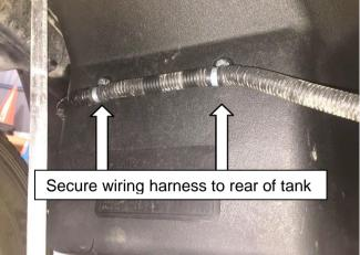
Attach wiring harness to the 2 M6 threads on the rear face of the Frontier tank. Secure using  $2 \times P$  clips and  $2 \times M6 \times 16$  bolts and flat washers.
