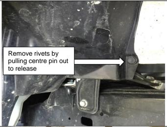
Remove the black plastic trims from the LHR wheel arch by first removing the plastic rivets.
