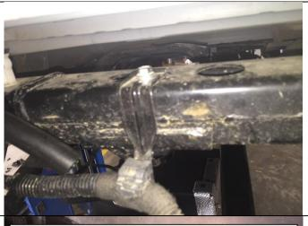
Remove the wiring harness mounting bracket from the top of the rear crossmember.
