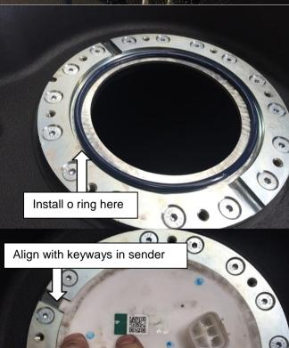
Install the o ring retained in the removal procedure into the groove in the fuel sender sealing flange.
