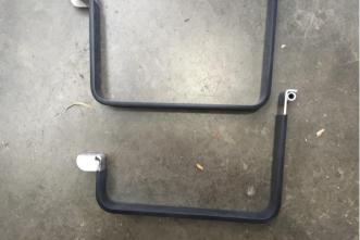
Install the rubber tank strap cover to the inside face of the mounting brackets as shown.
