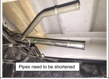
Locate and identify the 2 steel breather pipes that need to be modified.
