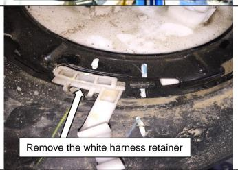
Remove the white wiring harness retaining clip from the fuel sender retaining ring.
