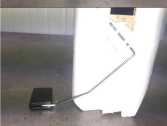
Bend the float arm down so that the bottom edge of the float is level with the bench top.
