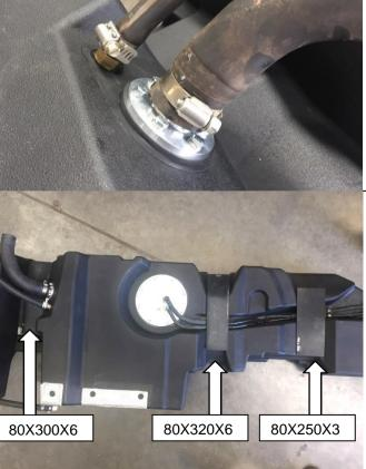
Install the rubber pads to the top of the tank. All 3 pads are different in size, install as per image on left.
