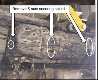
Remove 5 nuts securing tank shield and remove shield.
