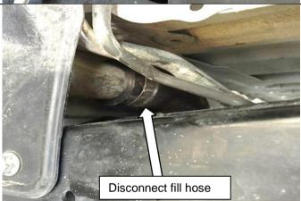
Disconnect the fuel filler hose from the steel filler neck. Retain the hose clamp for the installation process.
