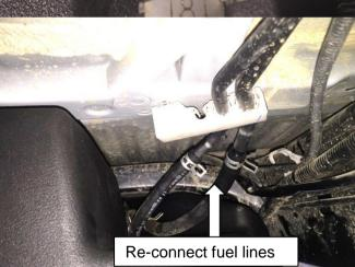
Re-connect the supply and return hoses at the LHF corner of the tank. Secure using the original clamps.
