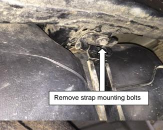
Position a jack underneath the fuel tank. Remove 2 bolts securing tank straps to vehicle. Retain the bolts for the installation process.
