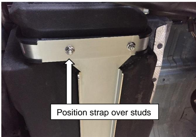
Position the rear mounting strap under the tank. Position the two holes in the bottom of the strap over the two M8 studs on the long mounting bracket.
