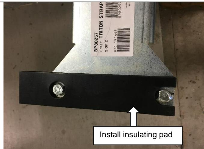
Remove the white protective backing from the 6mm thick self-adhesive rubber insulator. Install the rubber insulating pad around the two studs in the large mounting bracket.
