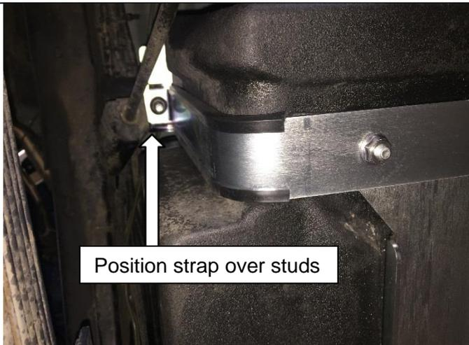
Position the rear mounting strap over the M10 studs in the rear mount bracket attached to the chassis earlier in the procedure.
