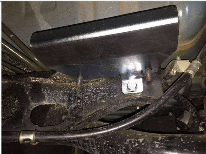
Position the front mounting plate over the two studs in the crossmember at the front of the tank.
