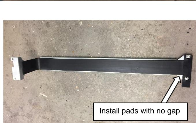
Remove the white protective backing from the longest section of 3mm thick self-adhesive rubber insulator pad.
