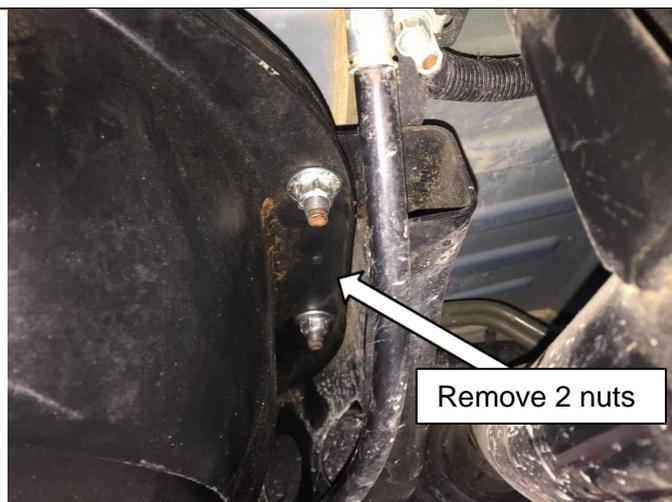
Remove the two nuts at the front of the tank.
