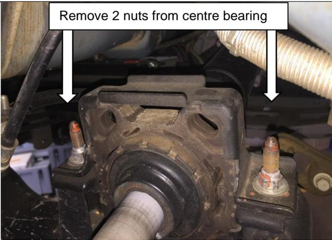
Remove two nuts securing the centre bearing to the chassis.
