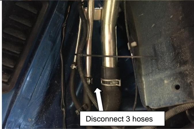
Disconnect the 35mm fuel filler hose, the 16mm breather hose and the 6mm rollover vent hose from the steel filler neck. Retain the hoses and clamps for the installation process.
