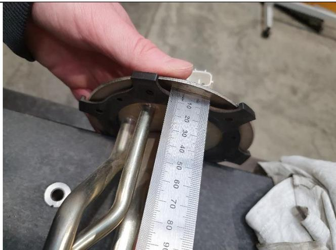
Once installed, the height from the underside of the sender top plate to the bottom of the fuel filter should measure 300mm on either version of fuel sender.
