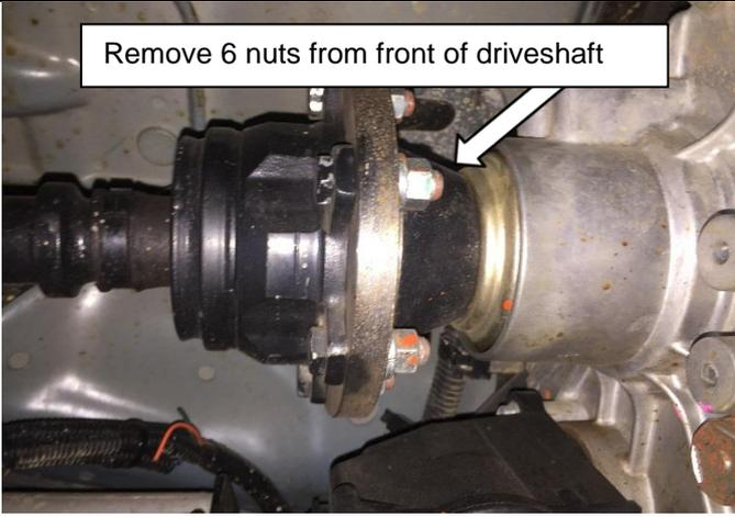
Whilst supporting the rear driveshaft, remove the six nuts securing the rear driveshaft to the gearbox output. Retain the nuts and washers for the installation process.
