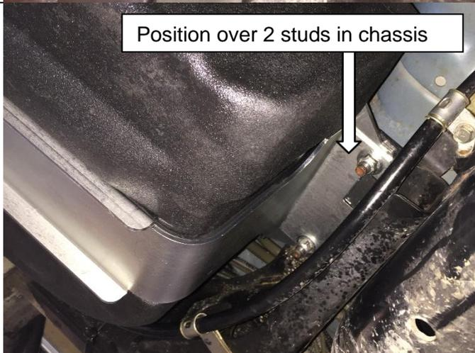
Continue to raise the tank into position. Position the mounting holes in the front end of the large mounting strap over the two chassis studs located at the front of the tank.
