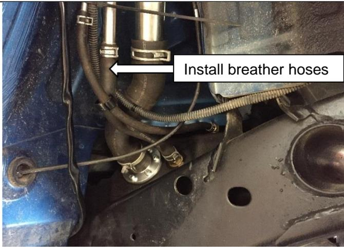
Shorten 16mm breather hose by 50mm and install into vehicle. Ensure that there is no low spot in the hose that can accumulate fuel. Secure with the clamps retained in the removal procedure.
