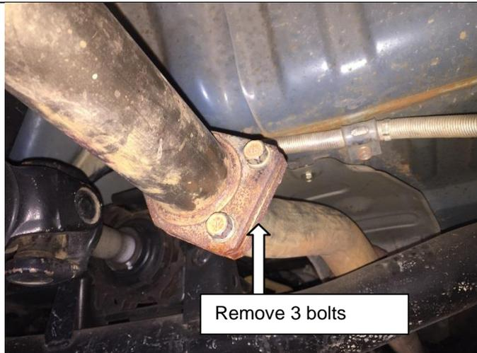
Remove the three bolts from the exhaust flange located near the centre bearing. Retain the bolts and gasket for the installation process.
