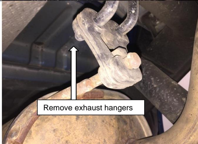
Whilst supporting the rear section of exhaust, disconnect the three rubber exhaust hangers by lubricating them and sliding them off the hook attached to the chassis.
