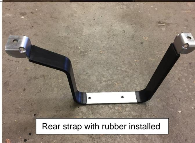
The strap should have rubber installed as shown.
