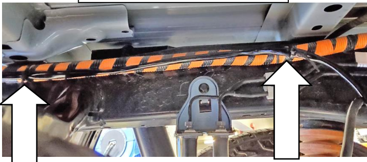
CABLE TIE LOOM ACROSS LEFT HAND CHASSIS RAIL
