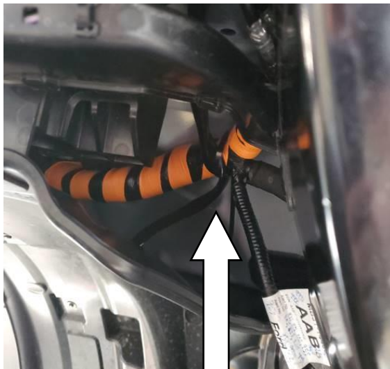
LEAD LOOM BEHIND LEFT-HAND FRONT WHEEL ARCH LINER
