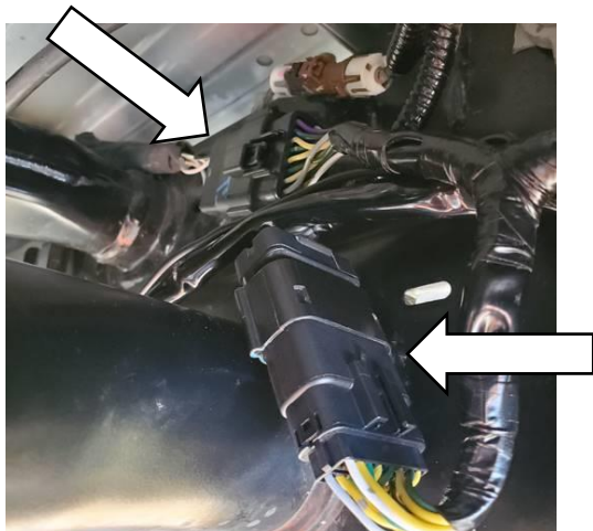
CONNECT LOOM TO VEHICLE'S CONNECTORS
