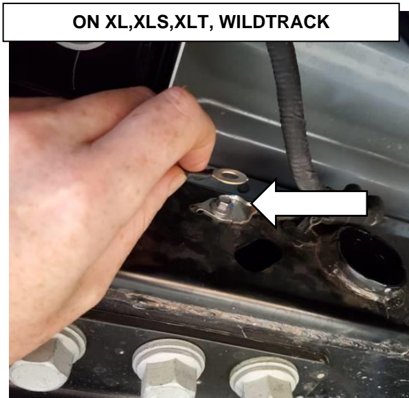
FASTEN EARTH TERMINAL TO M6 SCREW ON CHASSIS
