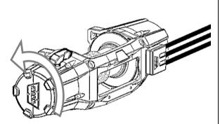
Warn Zeon winches\*: Undo the screws in the gearbox end of the winch. Carefully slide the gearbox away from the winch only until it is able to rotate. Rotate the gear box anti-clockwise 72° and replace screws.
