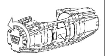
Warn VR Evo Winches: Undo the screws in the gearbox end of the winch. Carefully slide the gearbox away from the winch only until it is able to rotate. Rotate the gear box anti-clockwise 90° and replace screws.
