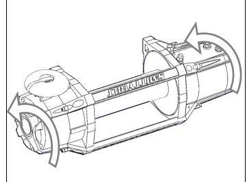
Warn / Magnum / Smittybilt winches: Undo the screws in the gearbox end of the winch. Carefully slide the gearbox away from the winch only until it is able to rotate. Rotate the gear box anti-clockwise 72° and replace screws.
