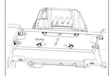
Carefully position the Control Box assembly in the winch recess, sliding the front of the mount plate under the winch recess lip.
