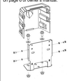
24. Carefully position the Control Box assembly in the winch recess, sliding the front of the mount plate under the winch recess lip while passing the control box cables through the cut-out in the mount plate and between the mount tabs on the RHS of the bar. Align the 2x mount tabs on each side of the mount plate to the two mount tabs on the bar and then secure using the 4x M6 fastener sets removed in Step 2. Route and cable tie the control box cables clear of the winch spool. Rear view shown.
