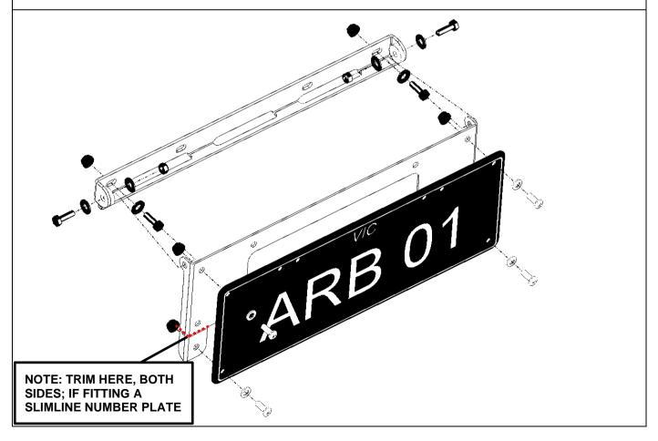
37. If fitting a slim line / "Euro" style number plate, trim on both sides at the dotted lines shown in the image above. Remove all burs and sharp edges using a file, then apply black touch up paint to the cut areas and allow to dry.
