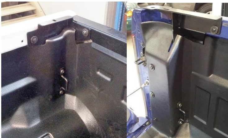
Bed liner hardware LH rear corner mounting bracket.
